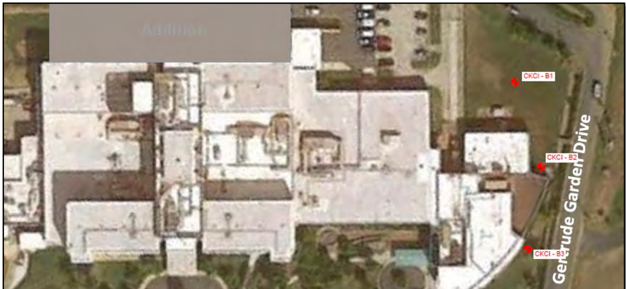
Figure 2: Approximate Boring Locations
